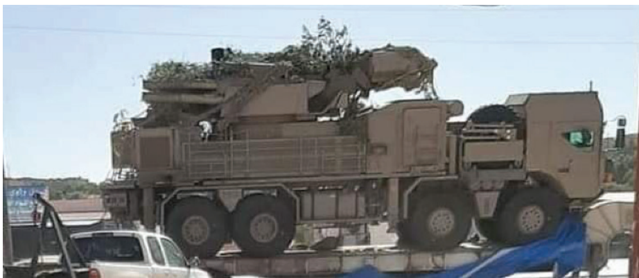
OSINT piece of evidence showcasing the Pantsir deployment in Libya. The picture was harvested from social media. The system is mounted on a MAN SX45 8X8 truck which remains a unique configuration of the UAE
